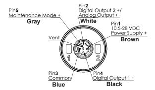
Note1: The TDEPD3, 4-20mA analog output is 3 wire.
