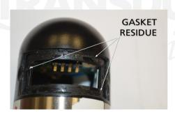
Remove paper backing from Gasket before installing battery. Install battery and press firmly all around battery door to insure a good seal.
